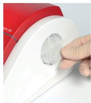
**STEP 2. Take out the used fan filter - replace with a new.**
