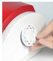
**STEP 1. Remove the fan filter cover.**
